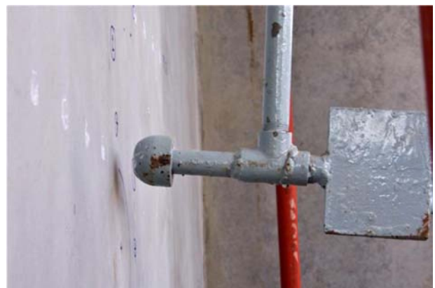
Figure 9: Impact test on a LiteCast panel
