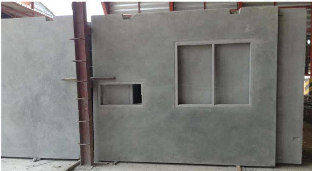
Figure 2: Customized precast concrete panels for housing
