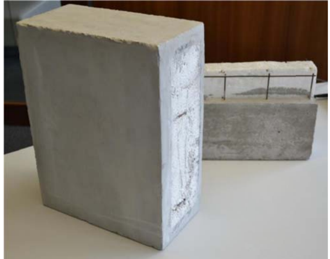
Figure 10: Transversal cut of a LiteCast panel
