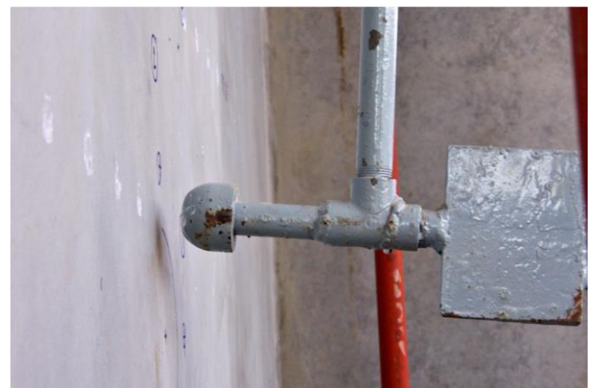
Figure 9: Impact test on a LiteCast panel
