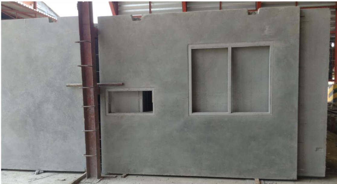
Figure 2: Customized precast concrete panels for housing
